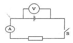
The voltmeter, V and the ammeter, A readings in the circuit above when switch S is open are 3.0V and 0.0A and when the switch is closed are 2.4V and 2.0A. Calculate the internal resistance of the cell. (3 marks)
